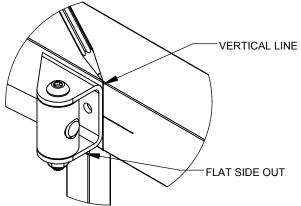
NOTE: The orientation of the gate bracket must be correct in every step.
