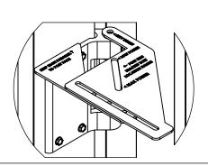
**3A** - Place post bracket over or under the template and flat against the post.
