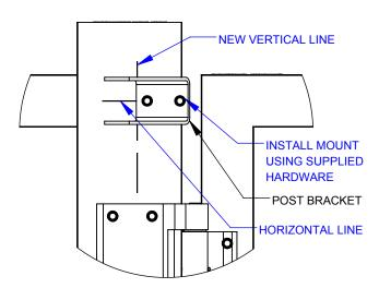
**7** - Center post bracket over the horizontal line made in step 1C and next to the new vertical line made in step 6. Ensure the bracket is level and mark hole locations. Pre-drill holes if needed and attach the post bracket to the post using the included hardware.
