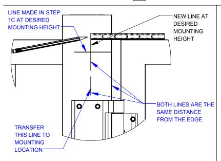
**6** - Measure to the location of the mark made in step 5 from the inside face of the post. Make another line at the desired mounting height using distance measured.
