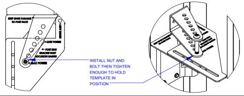
5 - Check to make sure the template and post bracket are still flat against the post and the hole is positioned correctly. Using a pencil, mark the post at the front (or back) edge of the post bracket as well as which hole the bolt is in.
